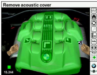
Fig. 10: Remove acoustic cover
